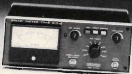
R310. Sinad-meter. 20 mV - 10 V. ±1 dB. 100 kohm. Millivoltmeter 10 mV - 100 V. 100 Hz - 20 kHz. 1.740:-
