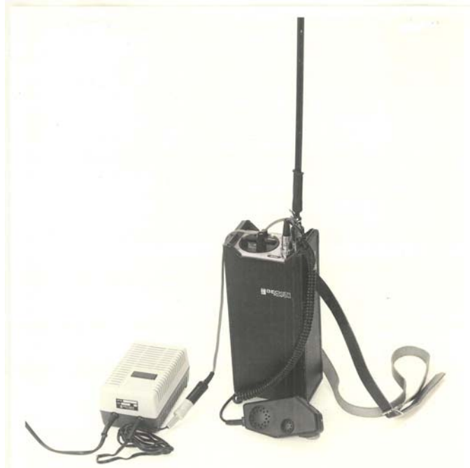
Radiostation RA-163 Foto FFV
