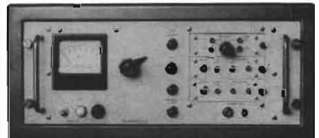
A typical Monitor in series 000 for measurement of Noise and Power.
