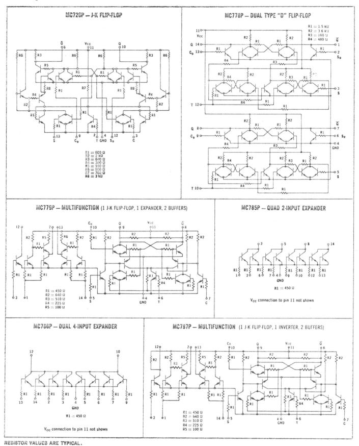
Integrated Circuits Schematic Equivalents MC788P - MC799P.
