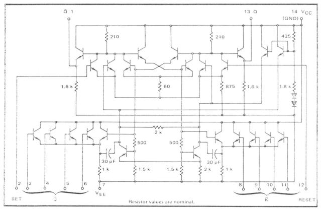
Integrated Circuits Schematic Equivalent CµL 9958
