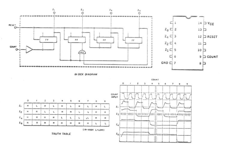
Circuit Block Diagram and Pin Number Functions  $C\mu L$  9958
