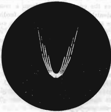
Fig. 21. Oscilloscope photograph of the B & K True R.M.S. rectifier characteristics as used in the Electronic Voltmeter Type 2409/2416. The same quantities are traced as in Fig. 19.
