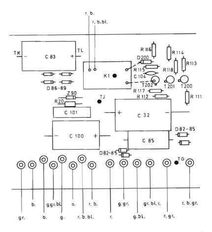
Mounting of the relay K1 onto the main PC-board Figure 18
