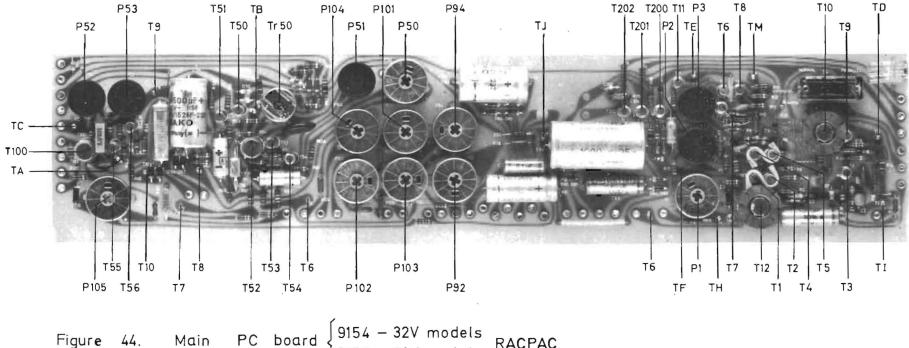
Figure 44. Main PC board  $\begin{cases} 9154 - 32V \text{ models} \\ 9155 - 60V \text{ models} \end{cases}$  RACPAC
