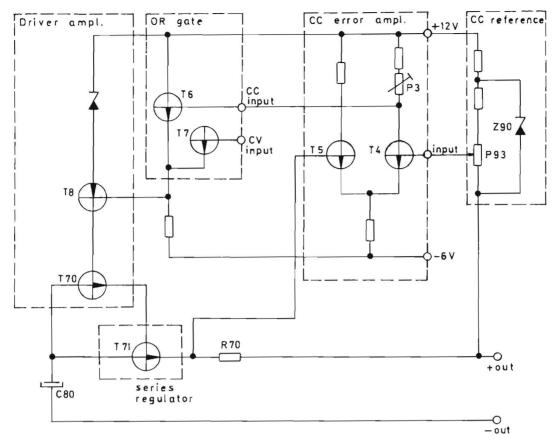
Principle drawing current stabilizing
