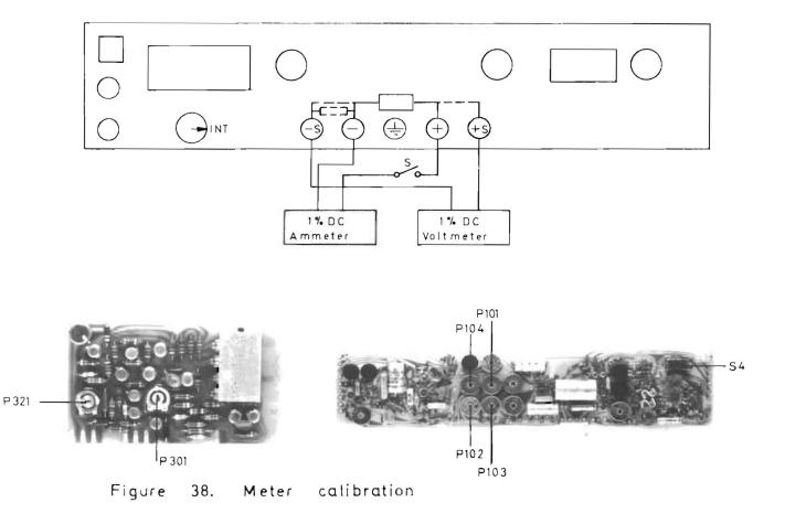
Voltmeter (Figures within brackets refer to 60 V models)
