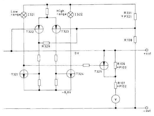
Voltmeter range selector circuit
