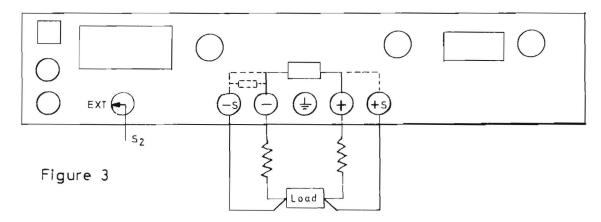
This circuit permits sensing the voltage at the load terminals instead of at the power supply terminals. Thus regulation loss caused by IR drops in the load leads is compensated for. The influence from the resistance in the "sense" leads is negligible as a low (a few mA) and almost constant current flows through these.
