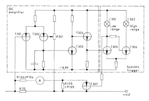
Ammeter range selector circuit
