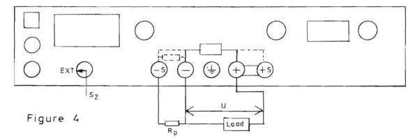
When the resistance programming mode is used, the output voltage is controlled by an external resistor. The connection procedure is as follows:
