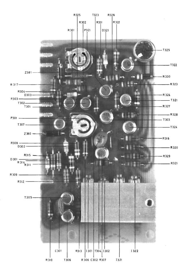
Figure 45. Lamp indicator PC board 9151 all models RACPAC
