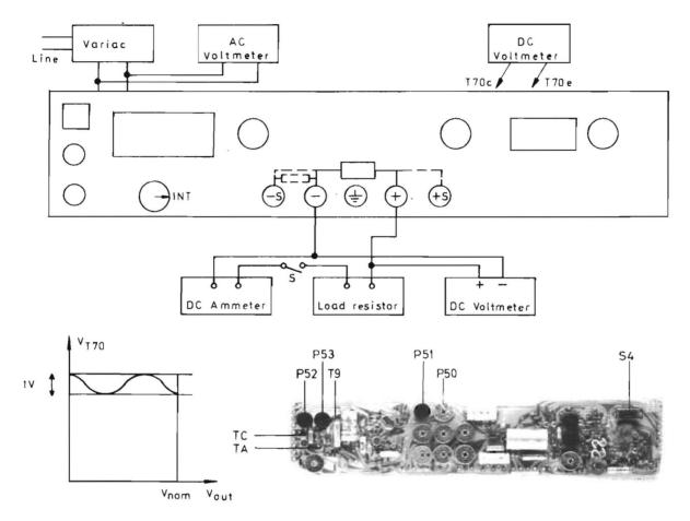
Firing circuit adjustment
