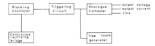
Block diagram of the firing circuit
