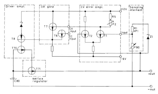
Principle drawing of voltage stabilizing
