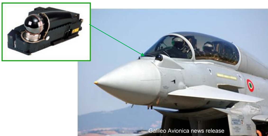
FIGURE 101. PIRATE IRST System on Italian Eurofighter. (The European PIRATE is one of a new generation of fighter IRST systems. Combined with long-range IR missiles, these devices will allow passive BVR attack.)
