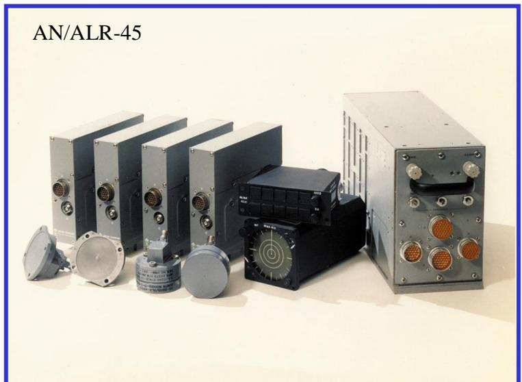
microcircuits using digital logic and clock drivers. From 1970 – 1974, the AN/ALR-45 was introduced to the Fleet.
