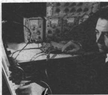
Power gain at high frequency being measured.
