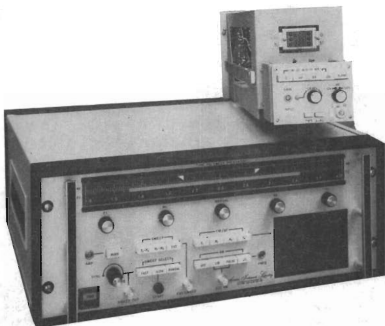
Plug-in sveposcillator 0,25 – 40 GHz
