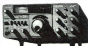
FT-225 RD: 2 m SSB/FM/AM, 0–25 watt 144–148 MHz. Digital. 5.595:–
