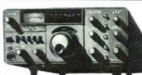
FT-225 RD: 2 m SSB/FM/AM. 0–25 watt 144–148 MHz. Digital. 5.595:–
