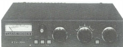
FV-700DM SYNTHESIZED EXTERNAL VFO/MEMORY
