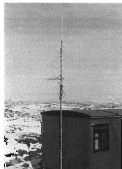
OX3VHF (GP60QQ) beacon: 50 MHz 20 W GP, 144 MHz 10 W 2x4 el.
