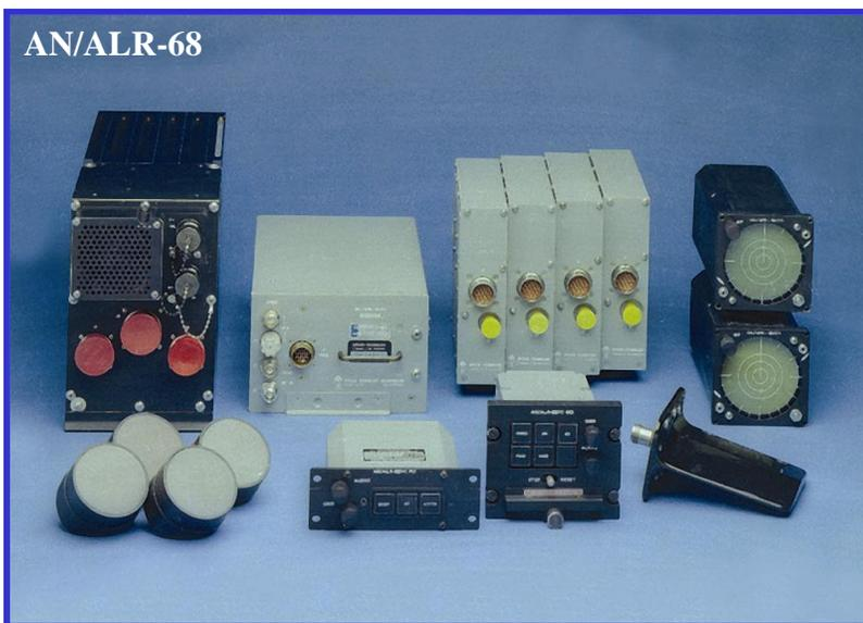
The Vector V signal data converter formed the basis of the AN/ALR-68(V), as well as the nucleus of the Enhanced Radar Warning Equipment used on the MRCA Tornado.
