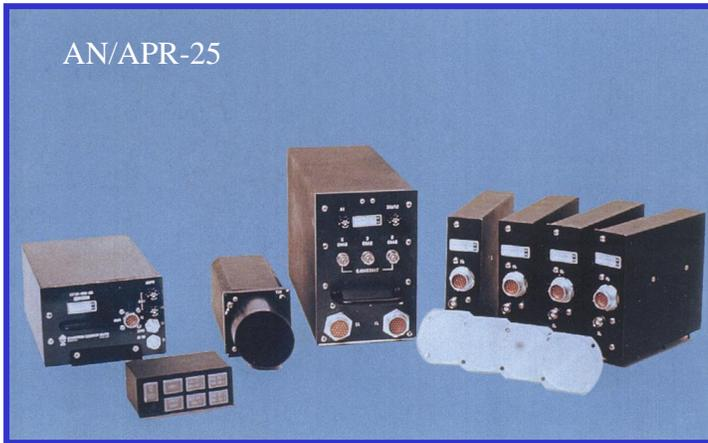
In November 1965, the USAF Sacramento Air Material Area awarded Applied Technology a contract for 500 AN/APR-25s, the system nomenclature for the Vector IV concept. The system was based on the use of crystal-video detection techniques in the threat bands only, where the hostile equipment's relative direction was resolved by a CRT display using vectorial inputs from four antenna patterns. Thus, the initial concept name, Vector IV.
