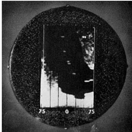
Figure 2-55.--A scope presentation of the APS-4 when set for the 20-mile range. The dark area represents a bay while the light area represents the land on either side. Note the surface ship targets in the convoy proceeding up the bay.
