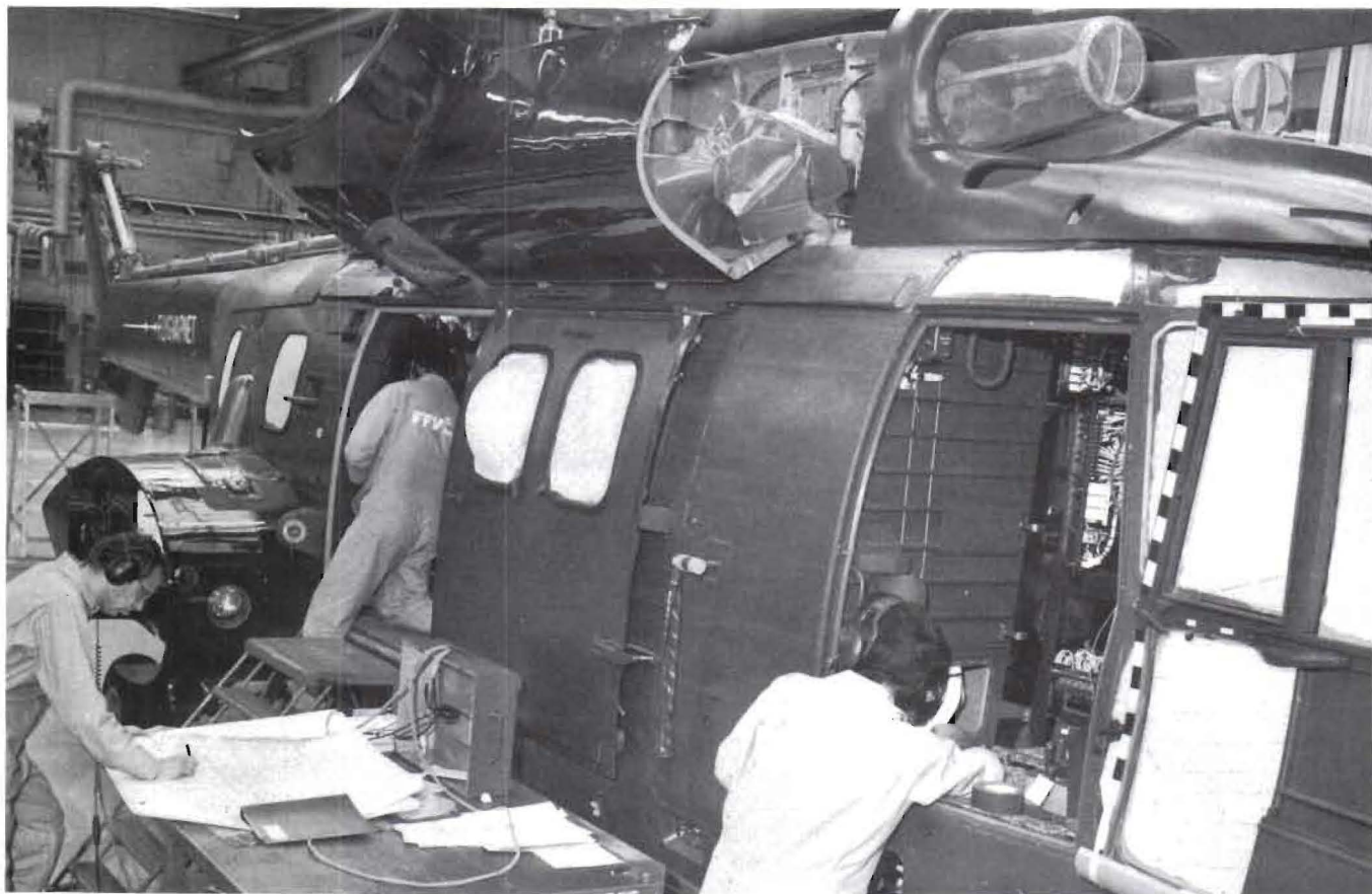
Här genomförs en "pin to pin check" (uppringning). Mer än 30000 anslutningar ska kollas. Here, a pin-to-pin check is being made. Over 30,000 connections have to be checked.
