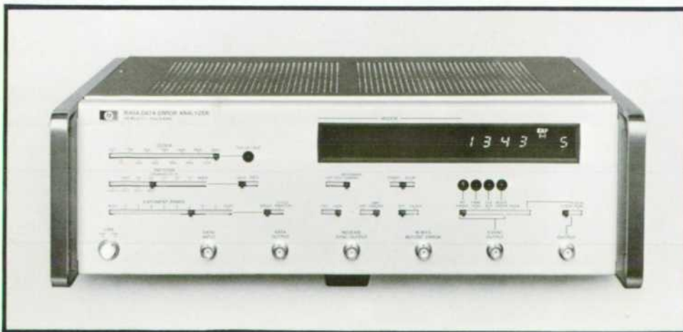
Fig. 1. Model 1645A Data Error Analyzer generates digital test patterns in its transmitter section, transmits the patterns through a communications channel, and analyzes the received patterns in its receiver section by comparing them to locally-generated patterns. It analyzes the patterns six ways simultaneously.
