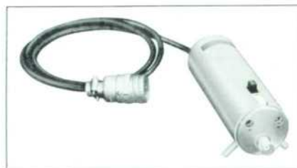
Fig. 6. Noise diode probe has excess NF of 5.2 db and is arranged for use with 30- and 60-mc i-f systems.
