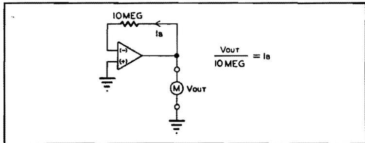
FIG. 2-8. 10MΩ Connection for Bias Current Measurement.
