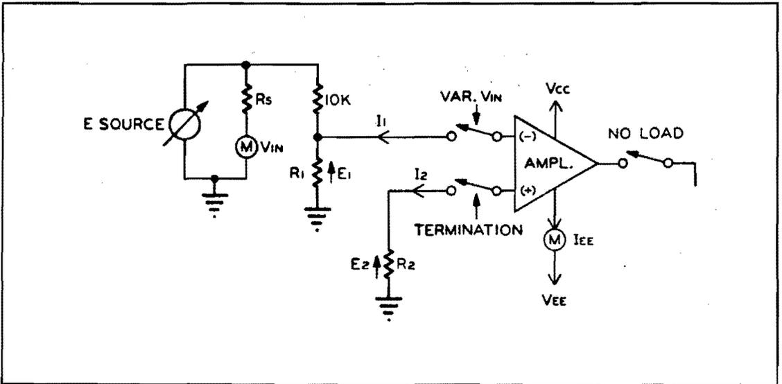
FIG. 3-6. Power Consumption: Test Circuit.
