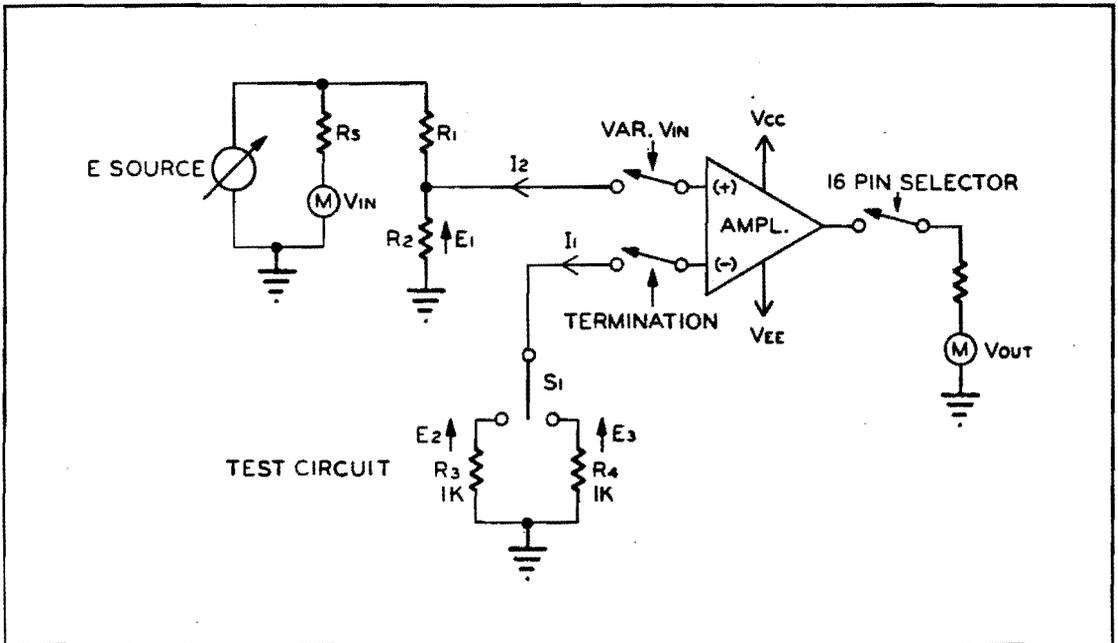
FIG. 3-2. Input Bias and Input Offset Current: Test Circuit.
