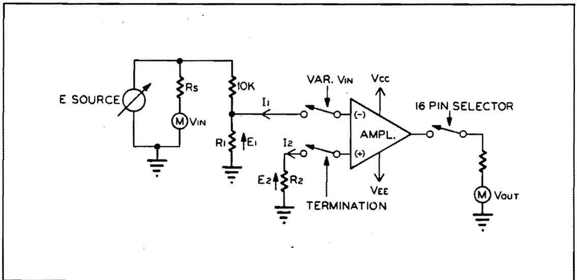
FIG. 3-1. Input Offset: Test Circuit.
