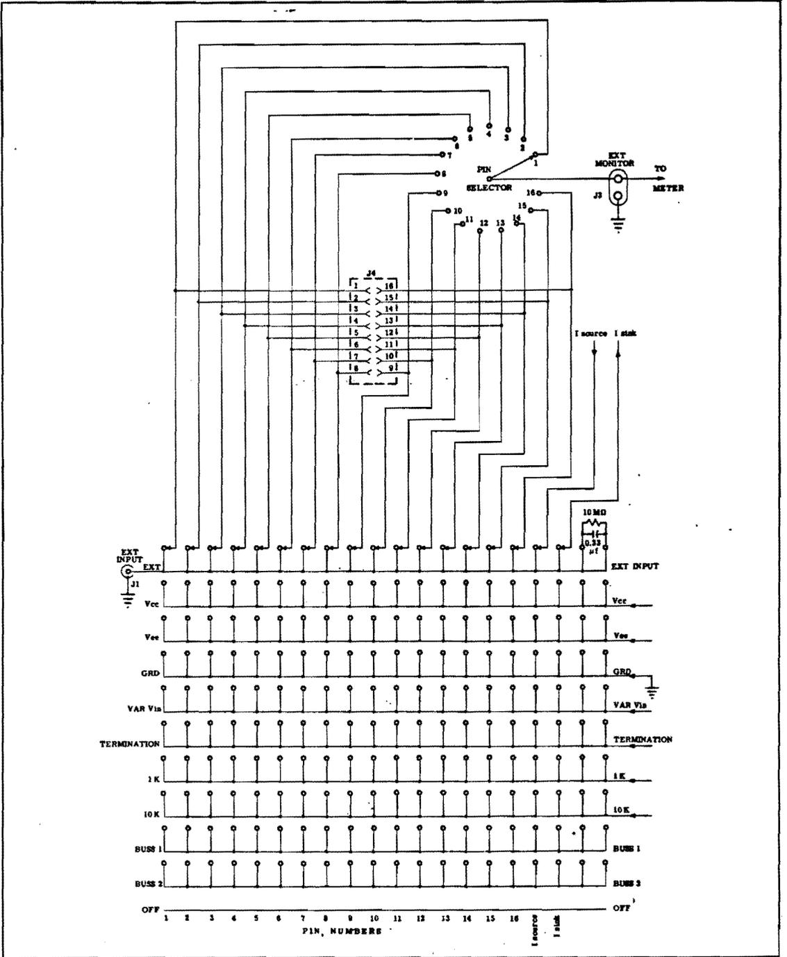
FIG. 2-2. Programming Matrix and Pin Selection Simplified Schematic Diagram.
