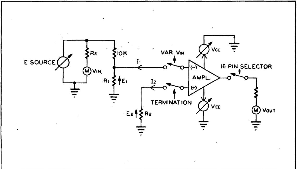
FIG. 3-4. Supply Voltage Rejection Ratio: Test Circuit.
