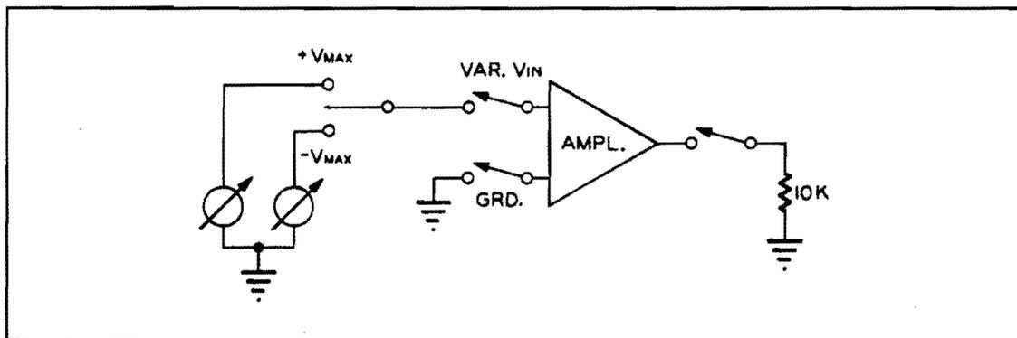
FIG. 3-3. Input Voltage Range: Test Circuit.
