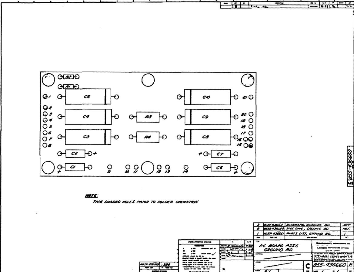
**CAPACITOR P.C. BOARD ASSEMBLY (A3) PARTS LIST**
