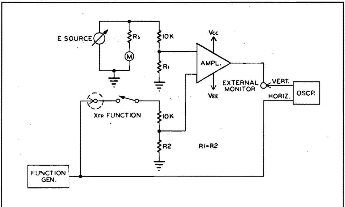
FIG. 3-7. Transfer Functions: Test Circuit.
