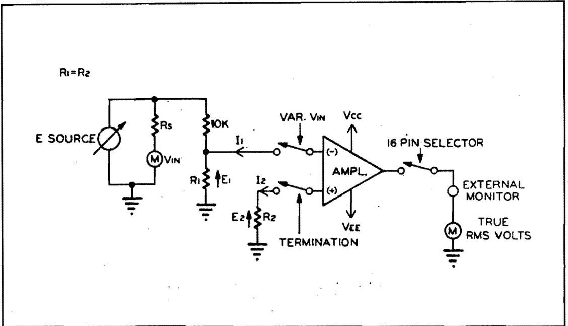
FIG. 3-5. Input Noise Voltage: Test Circuit.
