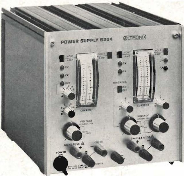
**LABPAC B 204 – A quadruple power supply especially for
