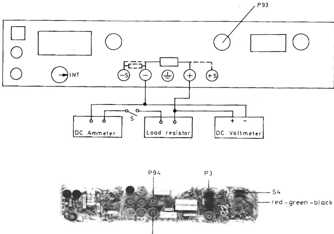
Figure 37. DC current limit adjustment
