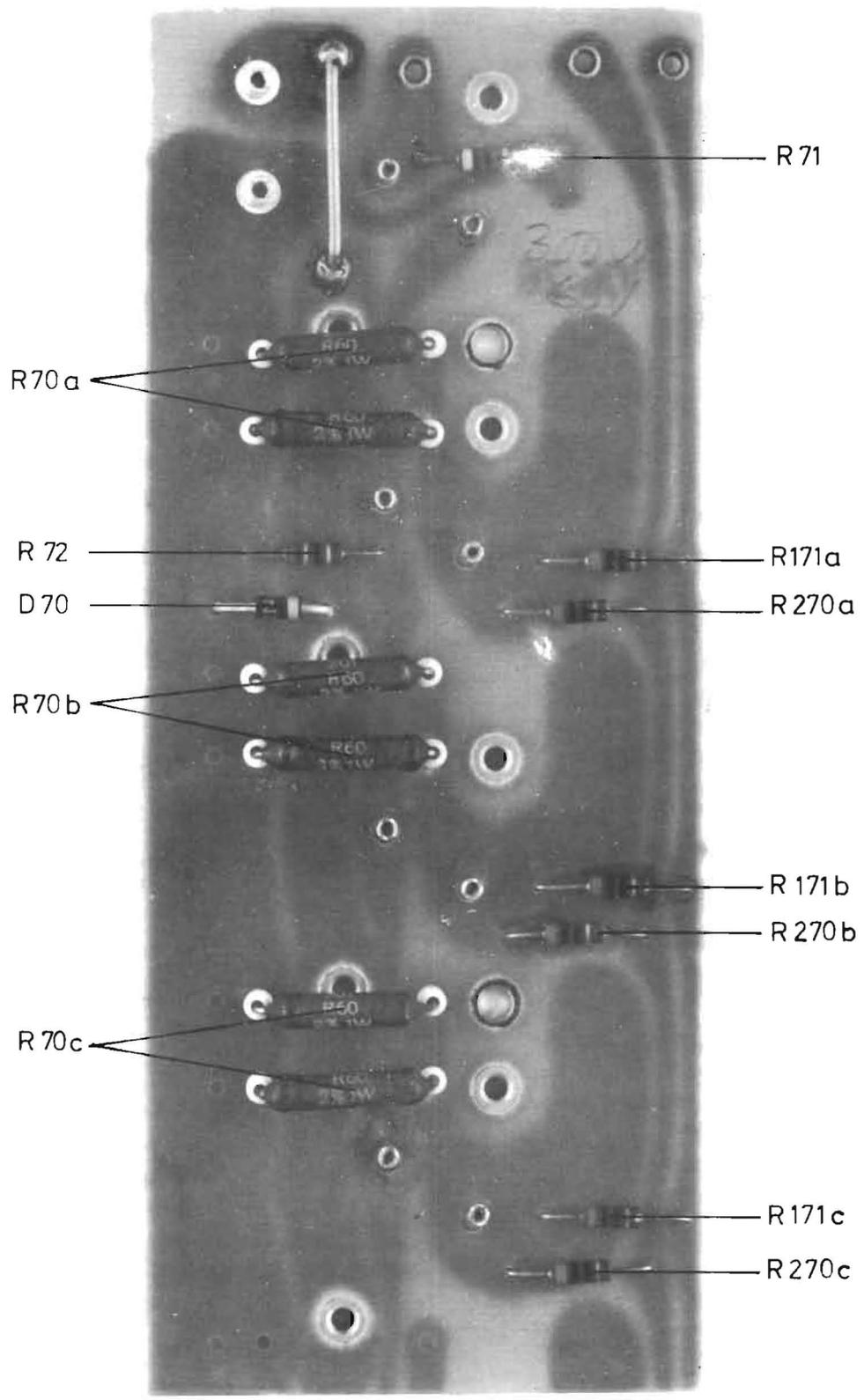
Figure 46. Series transistor PC board 9158 RACPAC 300
