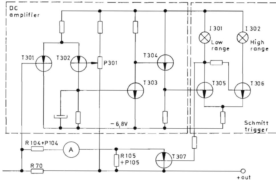
Ammeter range selector circuit
