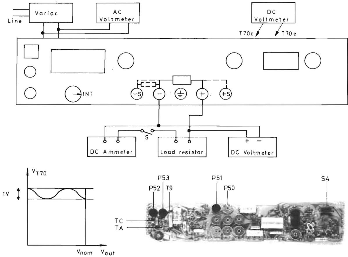
Firing circuit adjustment
