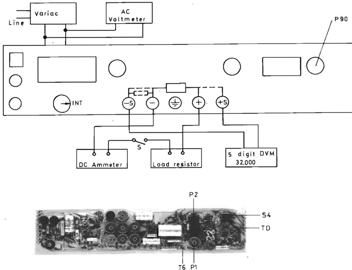
Figure 36. DC Voltage stabilizing calibration and specification
