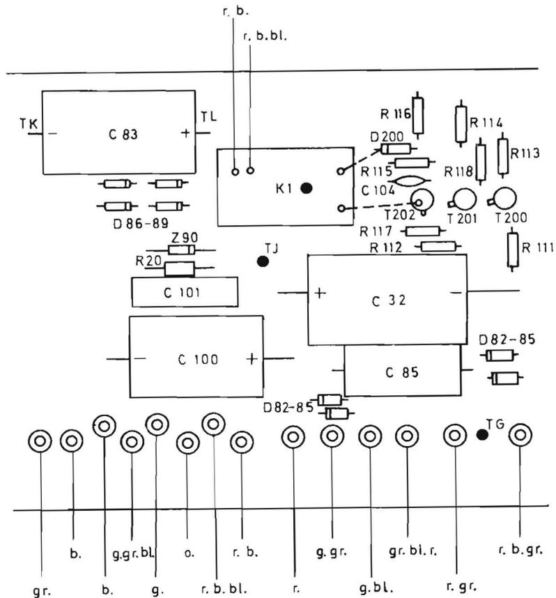
Mounting of the relay K1 onto the main PC-board
